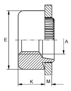
Female thread A = M2,5 Height K = 3.0 Outer diameter E = 6.0 Plate thickness = 5.0Recommended bore diameter +0.05 = 4.0
